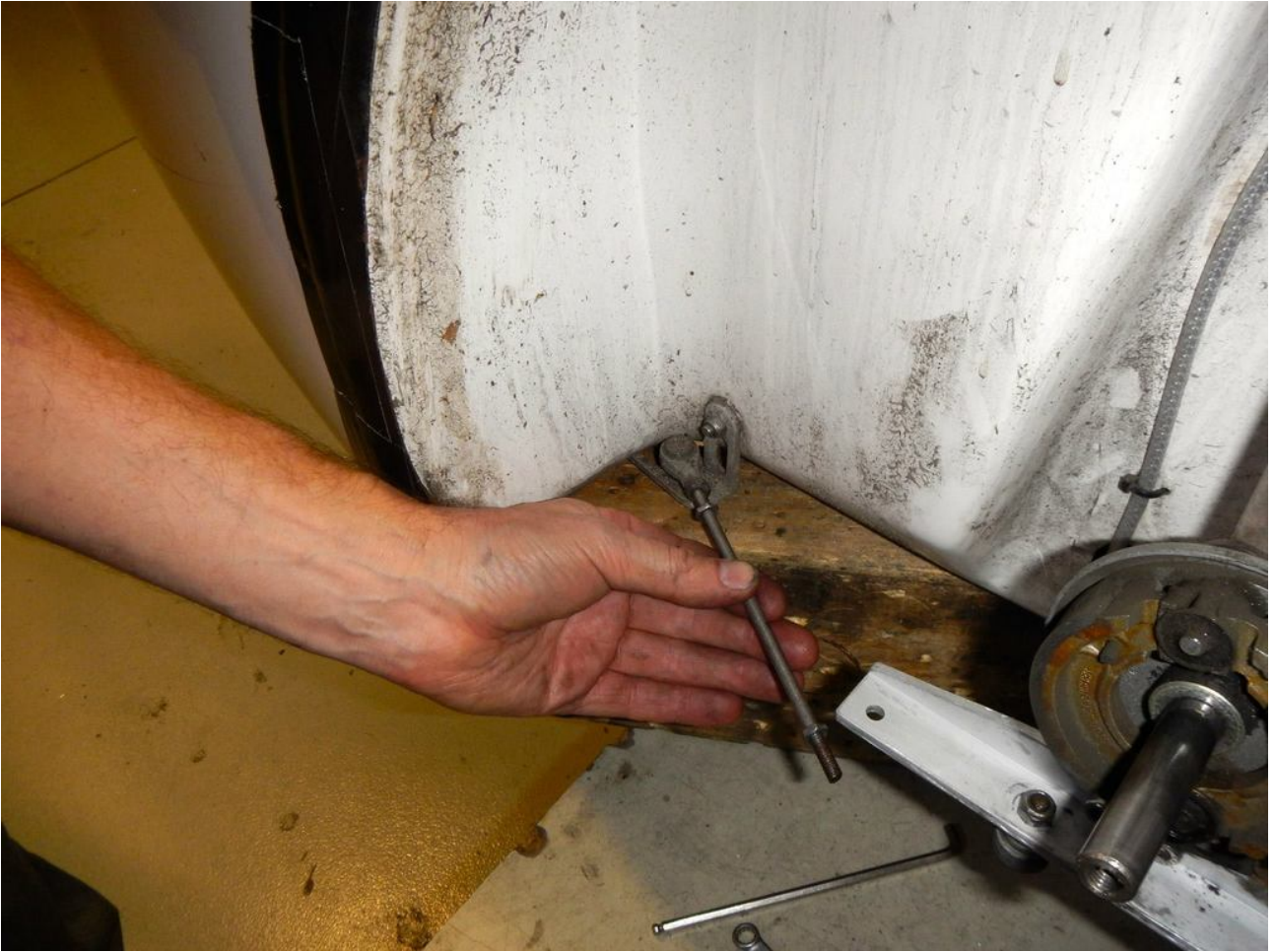
Illustration 29: Put the shortened rod back on.
