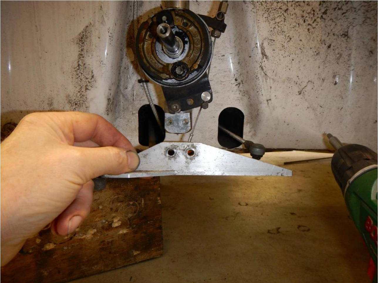
Illustration 4: Unscrew the steering plate from the suspension strut. The bolts are glued with loctite, so you may need to apply heat (heat gun) to get these loose.
