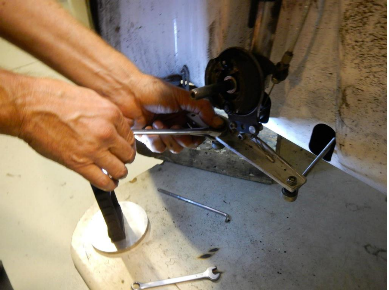
Illustration 22: Use a thin 8 mm spanner and a 10 mm spanner to tighten the nuts.
