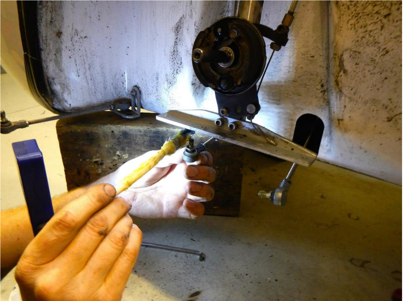
Illustration 19: Put a bit of grease on the ball joints' thread. Makes it easier to get loose the next time.
