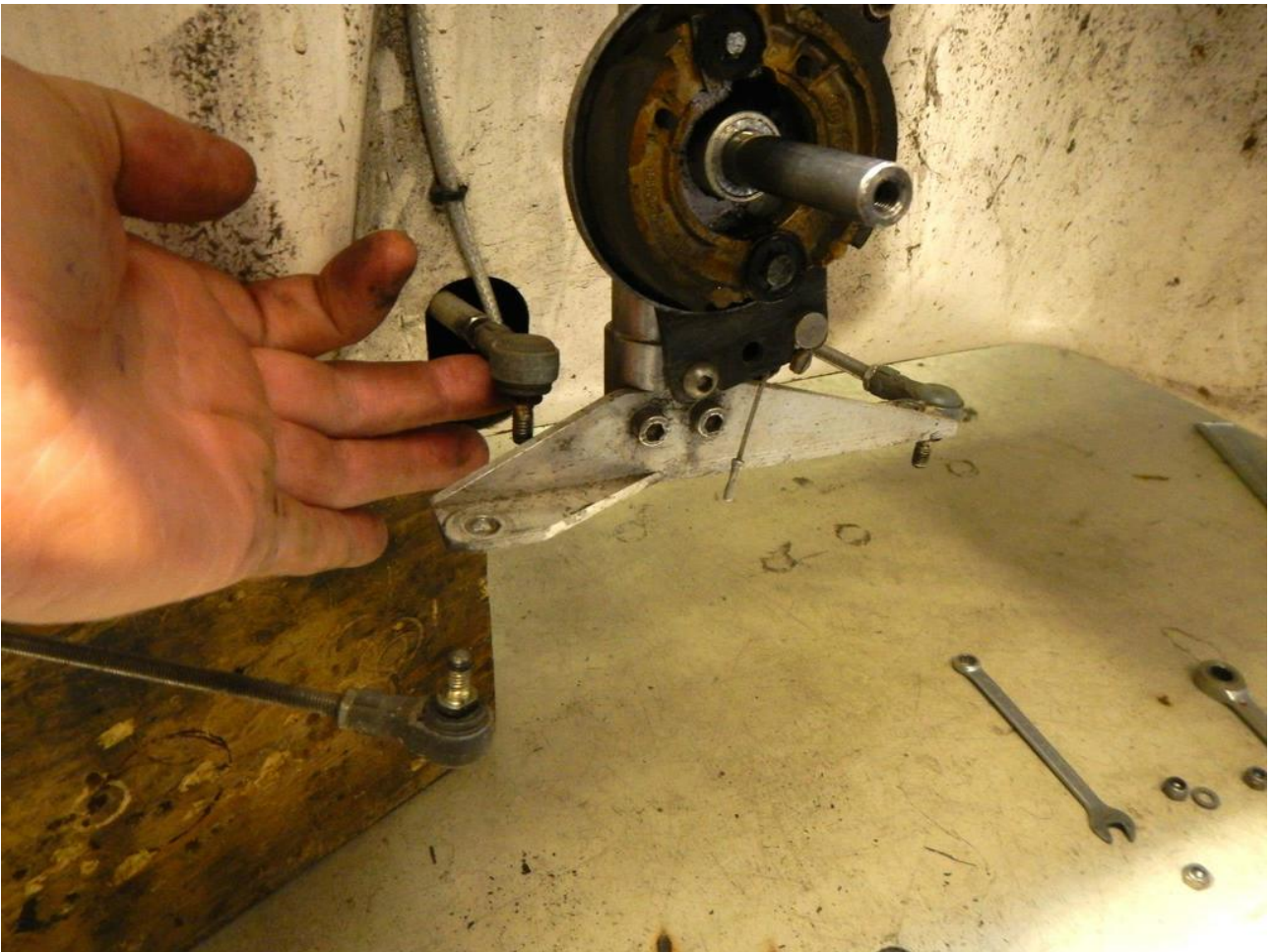
Illustration 3: Loosen all ball joints from the original steering plate
