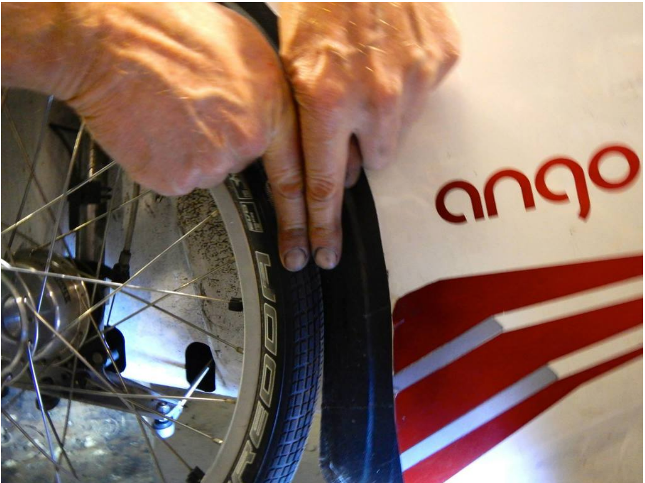
Illustration 33: The distance between wheel and wheel arch should be approximately the same on both sides of the arch.
