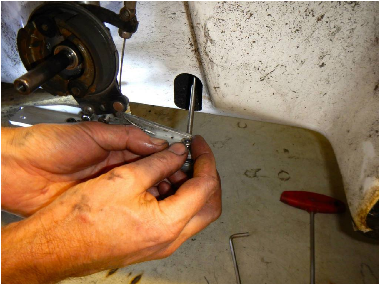
Illustration 21: Nuts go on top of the plate
