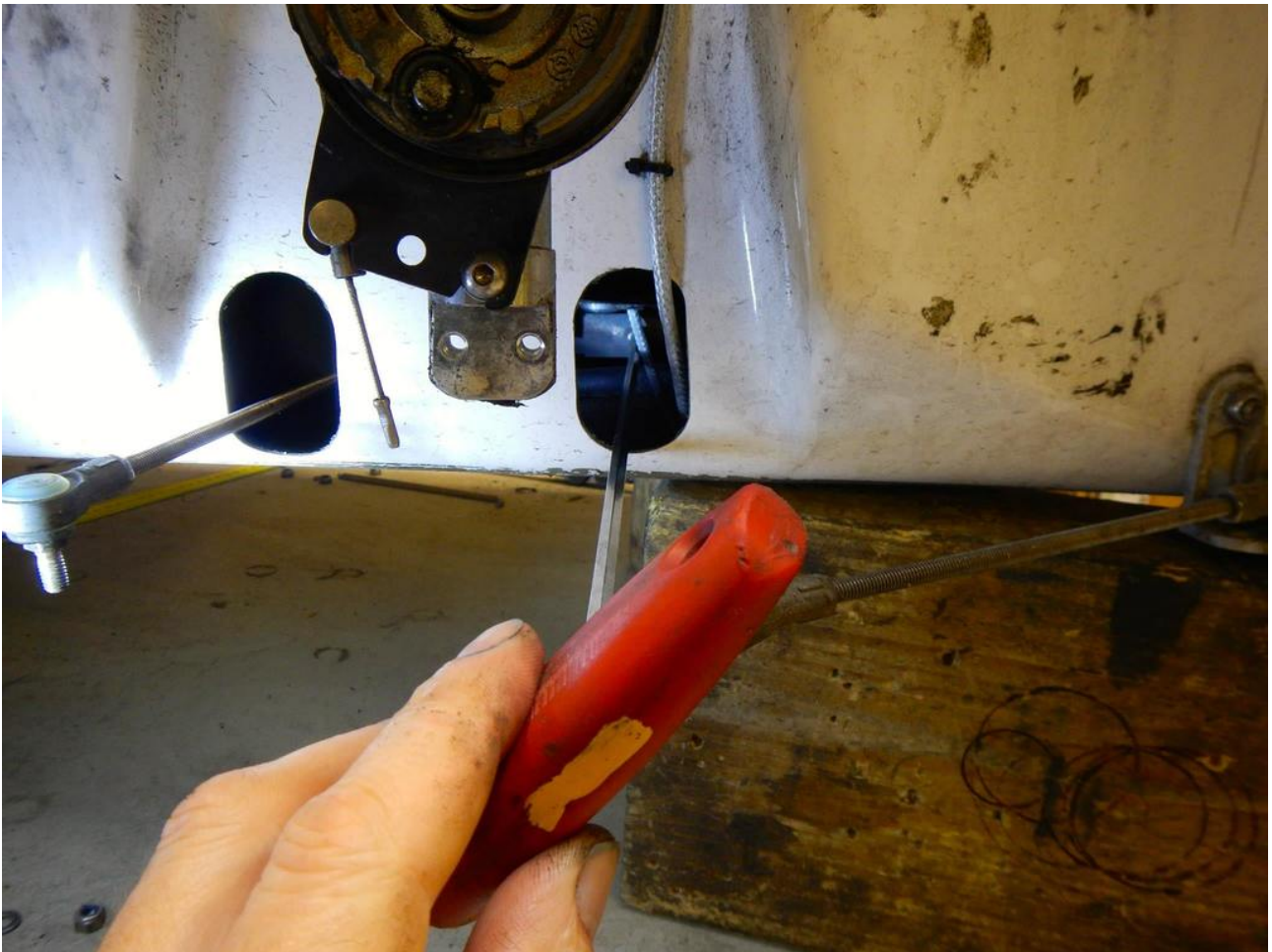
Illustration 9: Next is to loosen the clamp of the steering lever with a very long 5 mm allen key
