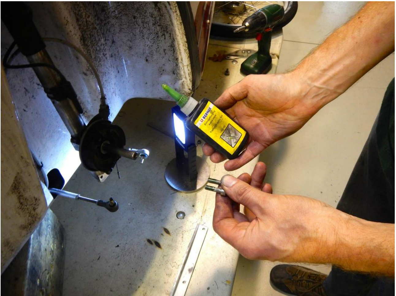
Illustration 17: It's time to fix the new steering plate. Use strong loctite on the thread, because this is a very important connection that you do not want to get loose while riding.
