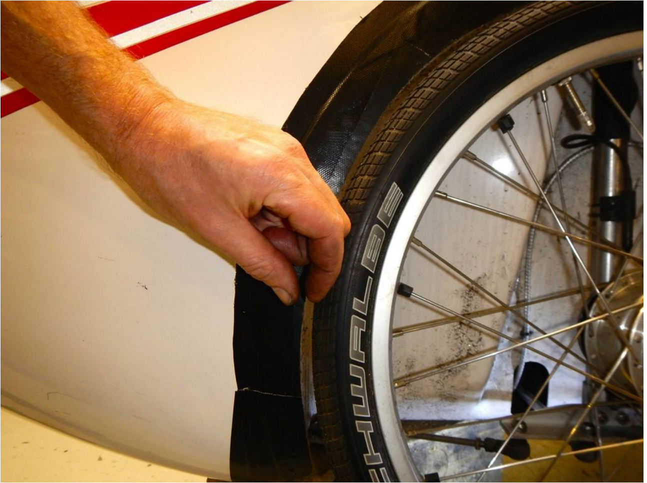
Illustration 32: Make sure the tire winds up in the center of the wheel arch. Adjust with the short rods.
