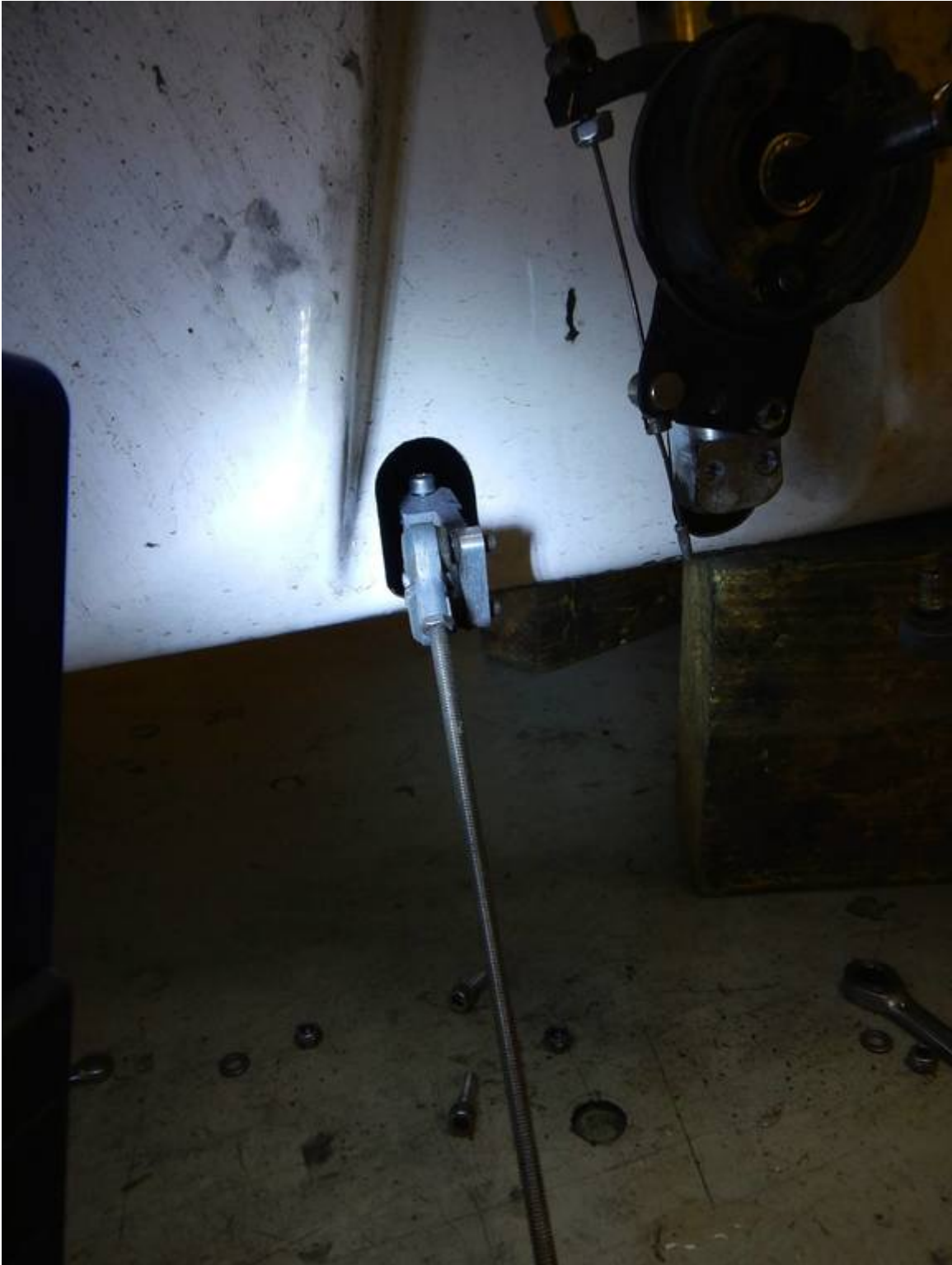
Illustration 10: Pull and twist the steer upwards while holding the steer rod. Then take out the steering rods with steering lever.
