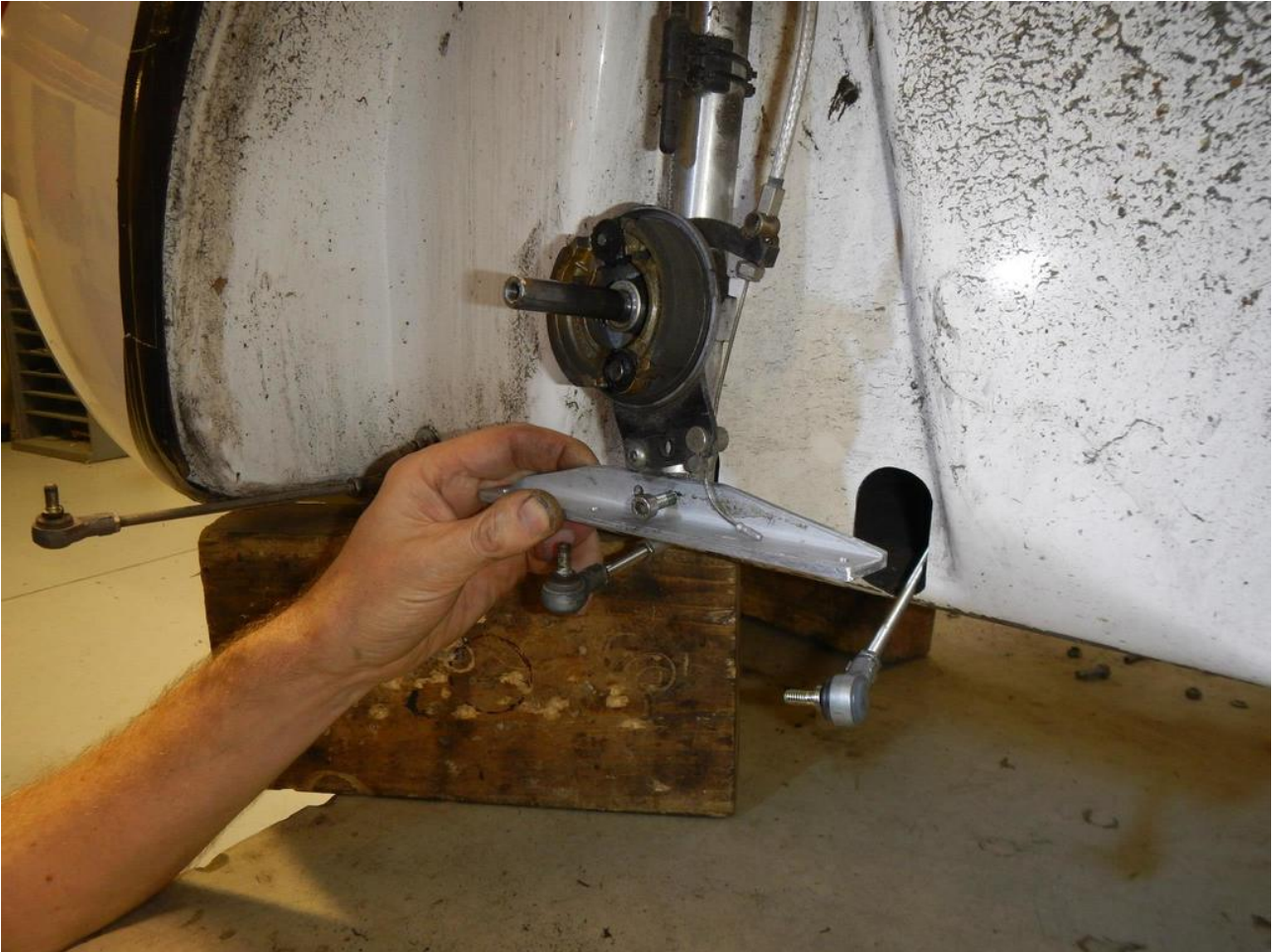
Illustration 18: Something I thought of later but not in this photo: Consider drilling a small hole in the steering plate to let the inner brake cable run through. Please, humor me.... it simply looks better and it nullifies the chances of the cable getting into the spokes
