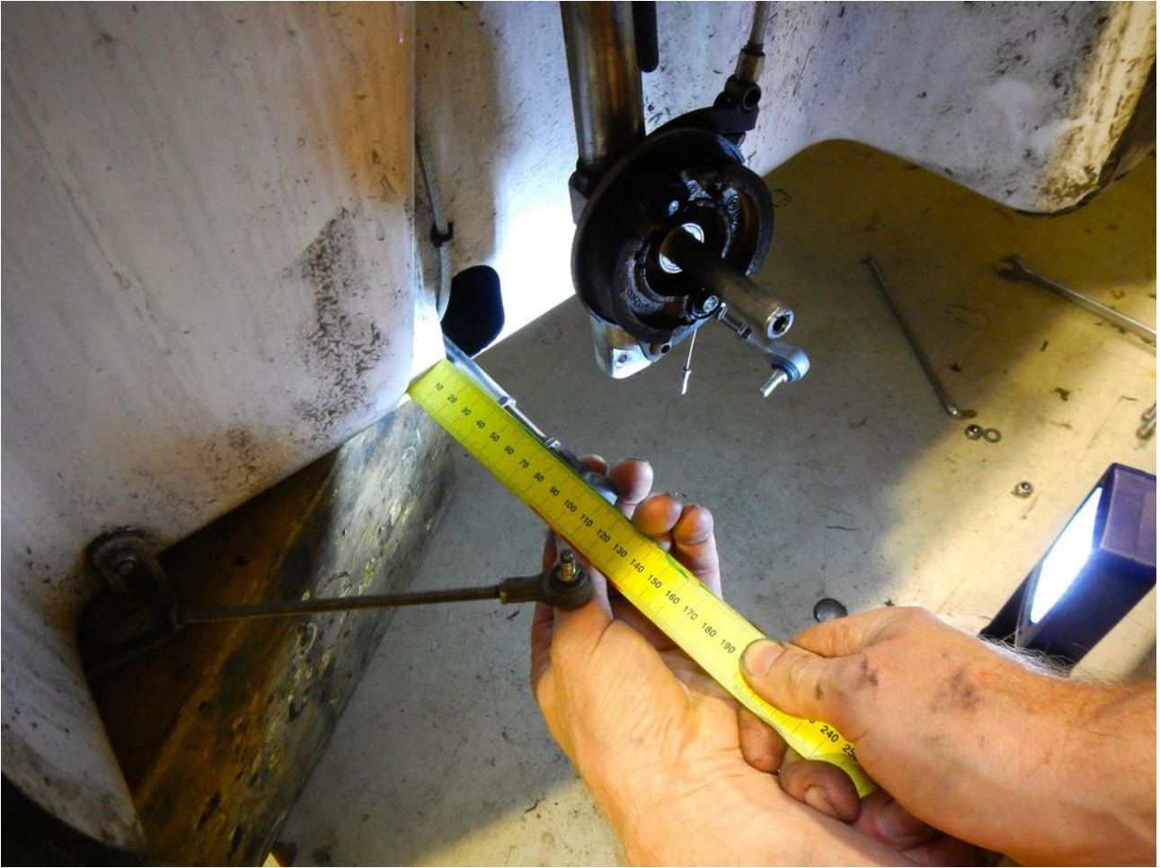
Illustration 13: 73 mm from the body to the start of the ball joint
