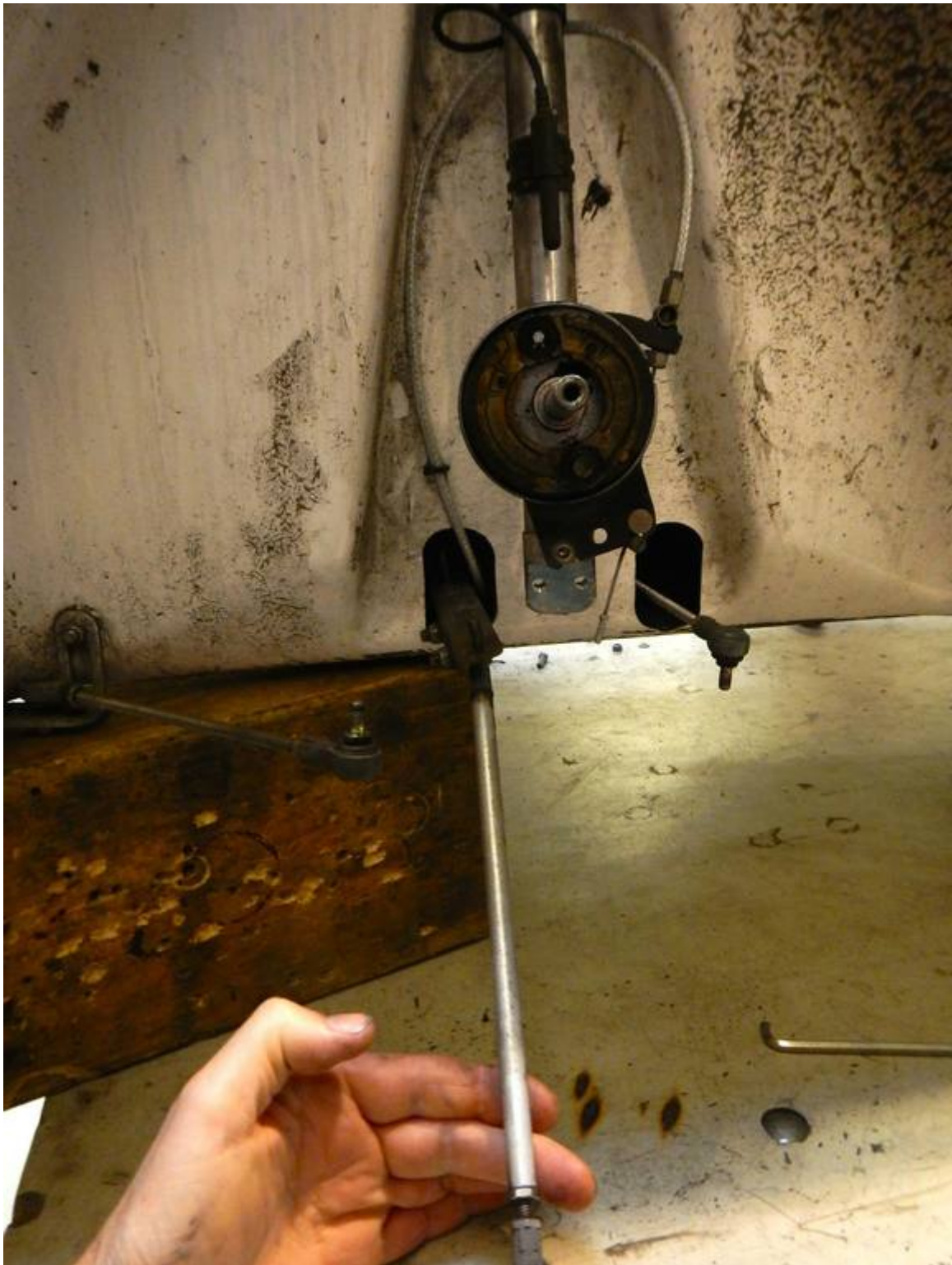
Illustration 7: Take out the anchor plate by pulling the rod sideways. A lamp makes it easier to negotiate it out.
