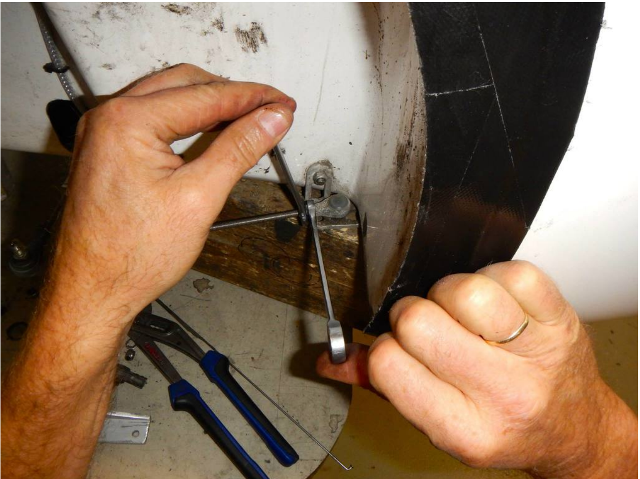
Illustration 30: Counter nut tightening. Watch out not to turn the ball out of the socket. That is why you need two spanners to tighten the counter nut.
