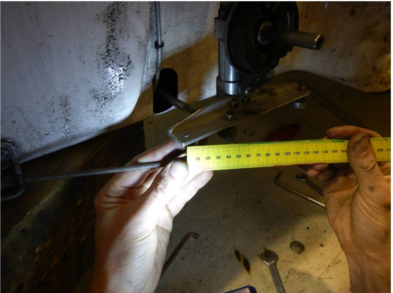
Illustration 23: The original short rods are too long. They need to be shortened.
